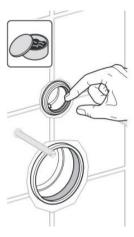
4. Connect the flush pipe and pan connector to the frame ready for connection to the toilet pan as shown, then screw the female threaded connectors (fixing bolts) onto the threaded bars so that the cut out aligns with the fixing hole in the toilet pan.
